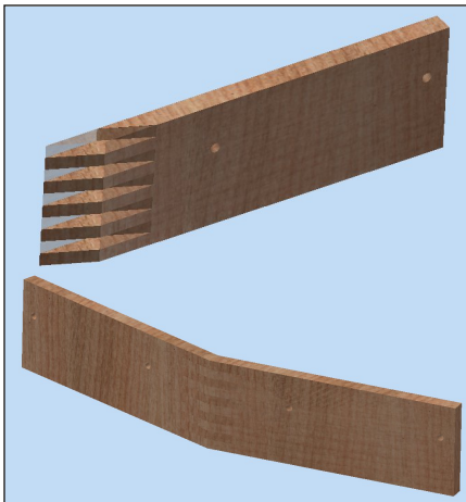
The wood on the hexagonal bumpers are joined with a box joint.
