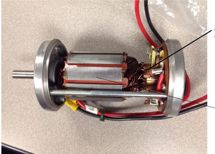
Comutator (switches direction of current)
