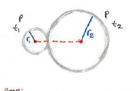
Notes about Gears: georboxes: gotten can have multiple reductions; you can keep gear distance the same if the solin of the teern stays the same gear terms: diametrial pitch (DP) is plinibler of teeth per inch of diameter, pressure angle (a) is angle between line of contact and common toingent
