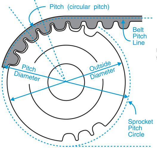
Belt pitch line and sprocket pitch circle match/are tangent for it to mesh
