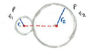
gear terms: diametrial pitch (DP) is planber of teeth per inch of diameter, pressure angle (a) is angle between line of contect and common tongent
